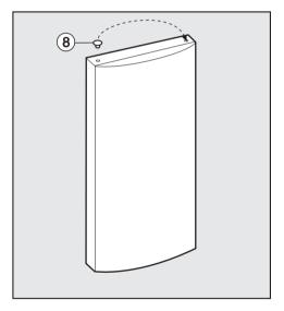
Remove cap ® from the bearing bush in the door and refit on the opposite side.
